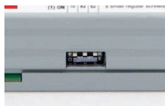
DIP switches allow the installer to select one of four operational modes.
