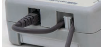
The strain relief helps prevent damage to sensor pad cords.
