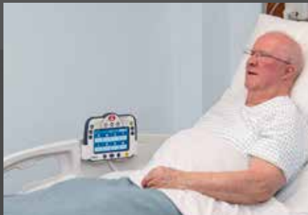
The device is powered and tethered at all times. When not in use, it can be placed into the holder, which can mount to most bed side rails.
